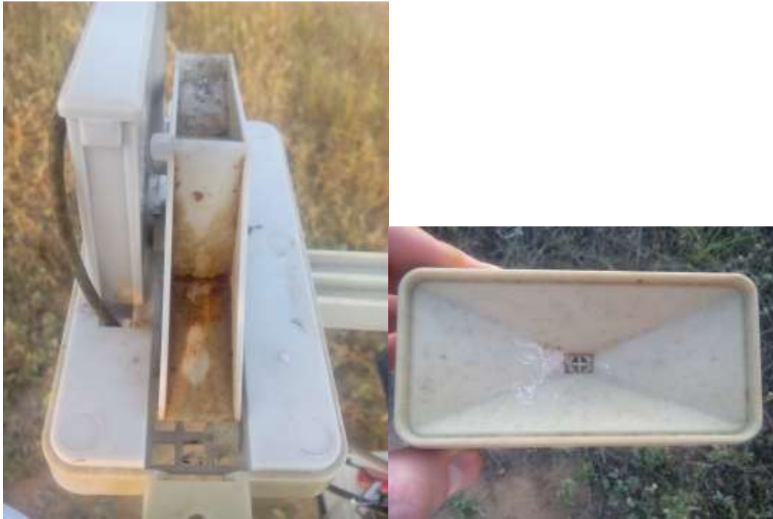
Figure 12: Original Raingauge after a year in the field
