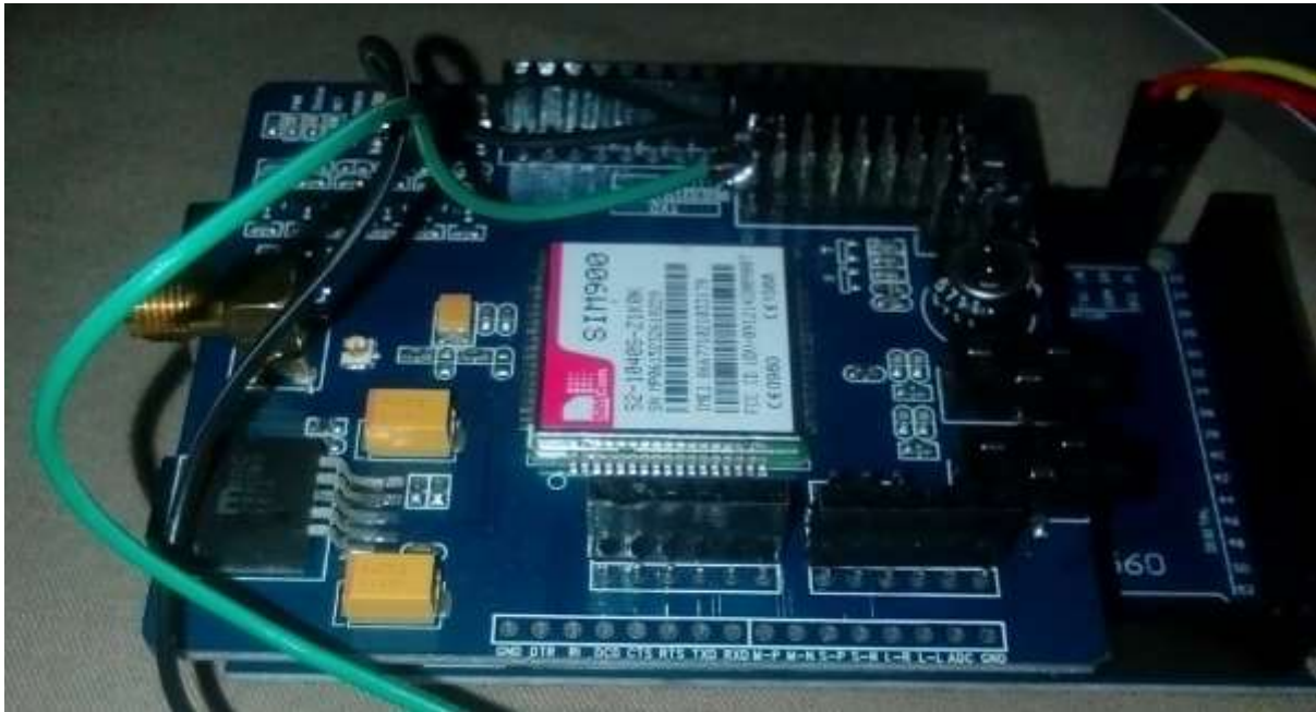
Figure 7: sim900 circuit board on the Arduino Mega (below)
