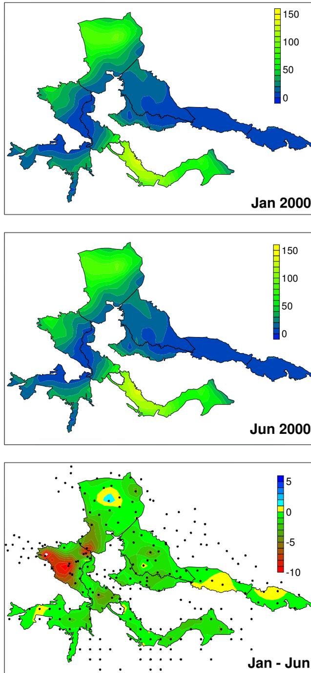
**Figure 7. Depth to groundwater (in meters) for the main irrigation systems in Zayandeh Rud Basin for January and June 2000 as well as the difference between these two months.**
