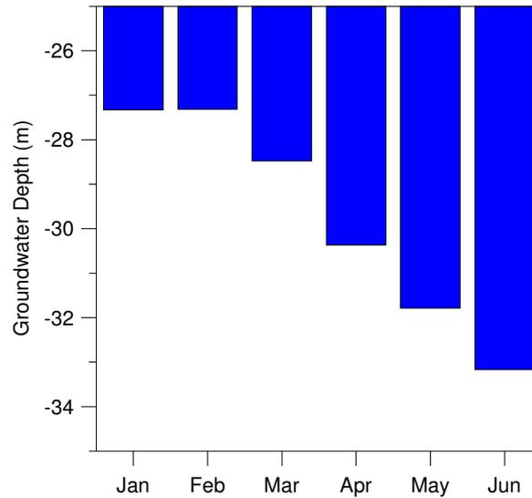
**Figure 9. Average groundwater levels for Nekouabad Left Bank irrigation system for January 2000 to July 2000.**
