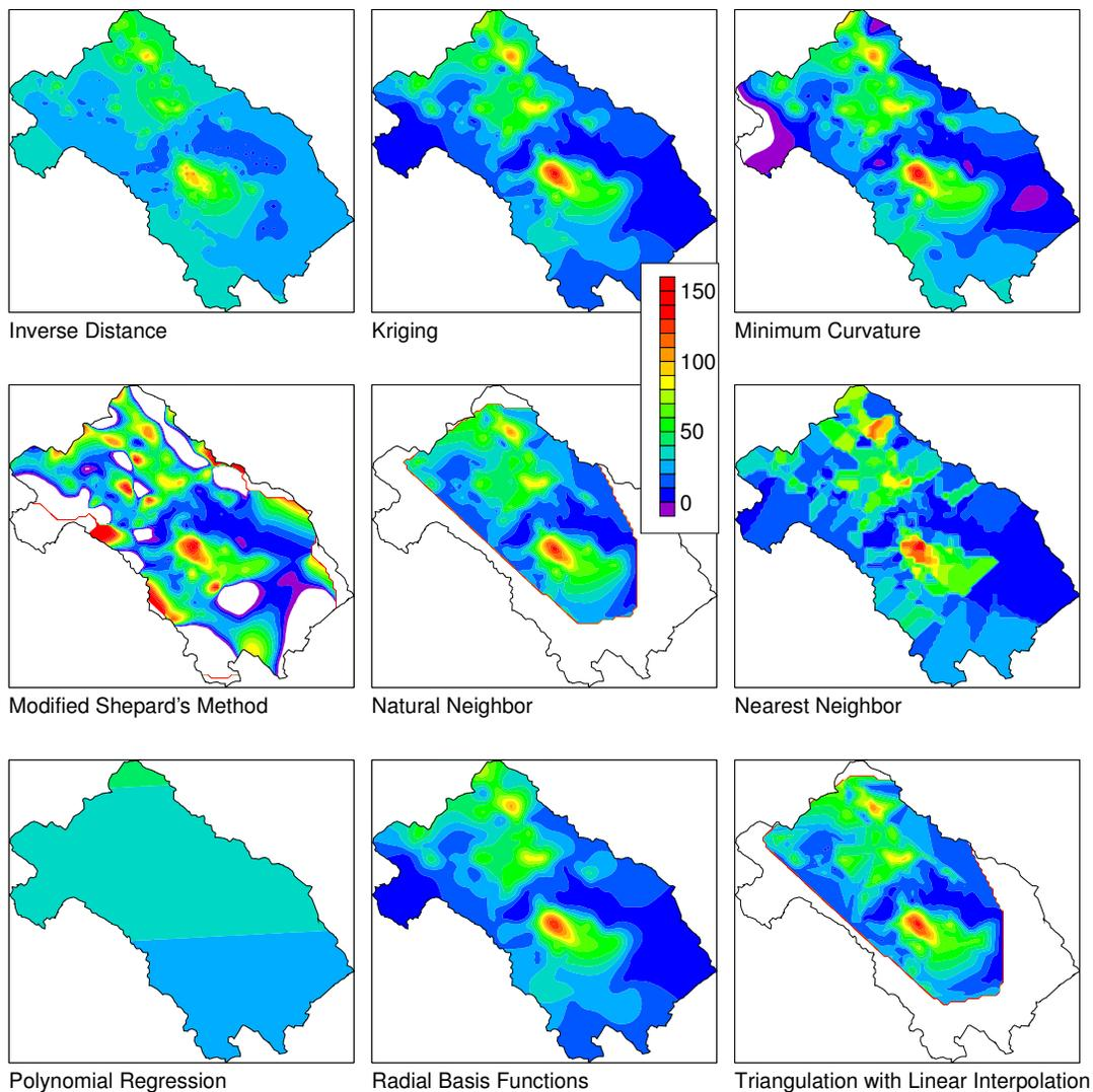
**Figure 3. Spatial interpolation techniques used to grid data for January 2000. Data represents depth to groundwater in meters.**
