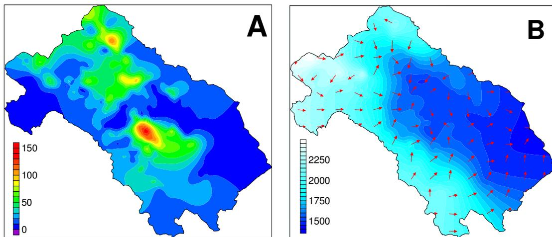
**Figure 6. Depth to groundwater (A) and groundwater levels (B) to a reference base (hydraulic head) for January 2000. All values in meters.**
