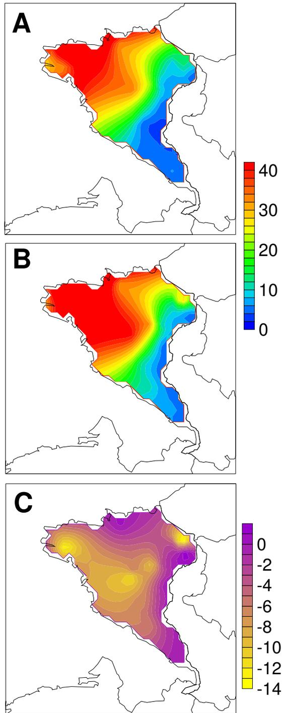
**Figure 8. Depth of groundwater level for Nekouabad-Left Bank irrigation system (in meters). Displayed are January 2000 (A), June 2000 (B), and the difference (C).**
