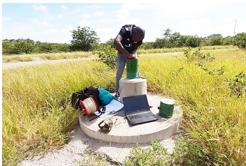
Downloading data in a monitoring borehole on the Tuli Karoo transboundary aquifer (photo: F. Ramusiya).
