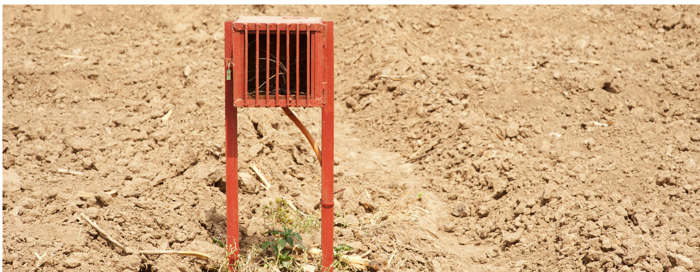
Data logger used for measuring soil moisture in Ghana (photo: Hamish John Appleby/IWMI).
