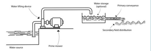
Figure 2.1: Typical water pumping system (FAO, 1985)
