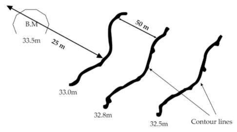
Figure 11.5: Using A-frame to map out contour lines
