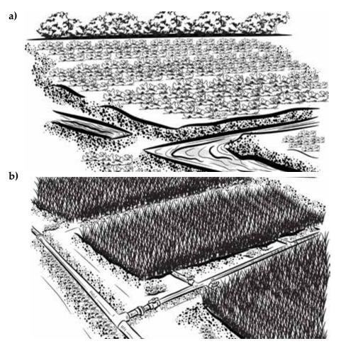
Figure 5.2: (a) Field channels for water conveyance (b) closed-pipe conveyance system
