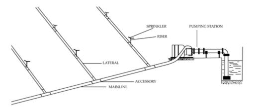
Figure 7.2: Different components of sprinkler system (Source: FAO, 1985)
