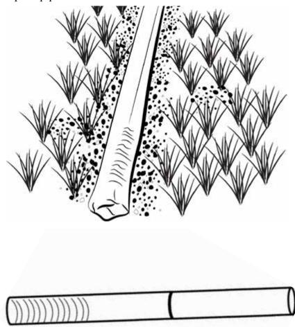
Step 3: Tube pipe – PVC with slots as screens
