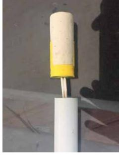
**Step 2** - Feed the sensor wire through the pipe.
