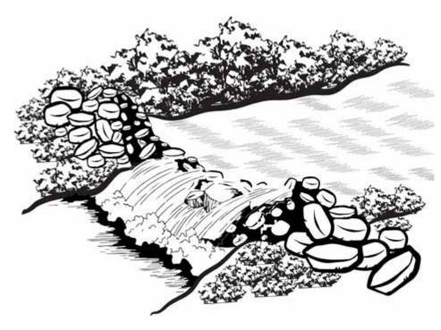
Figure 4.5: An embankment dam constructed from stone boulders
