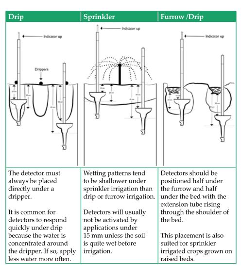
Figure 9. 4: Depth of placement of WFDs
