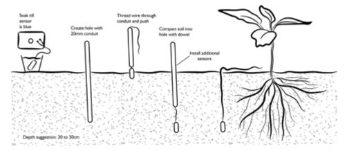
Figure 10.5. Installing single sensors
