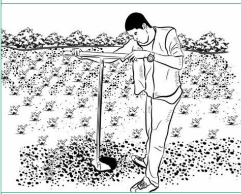
The detector is easiest to install using two augers: an auger (20 cm or larger in diameter) for the wide end of the detector funnel and another (5–10 cm in diameter) for the narrow end of the funnel. Alternatively, a spade and trowel can be used. Keep different soil layers separate when removing them from the hole if the soil type changes with depth. Installation is easiest when the soil is moist, rather than when it is very wet or dry.
