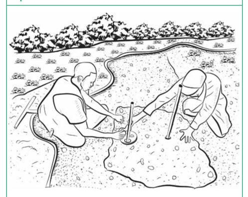
Pour the supplied filter sand into the funnel until it covers the locking ring by at least 1 cm. Lower the detector into the hole and measure the distance to the locking ring (or rim of the funnel) to check it is at the desired depth.
