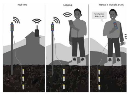
Figure 10.9. How the Chameleon Wi-Fi system communicates
