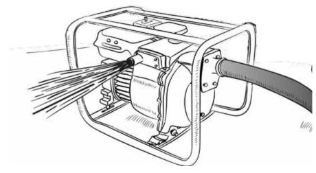
Centrifugal fuel-powered pump
