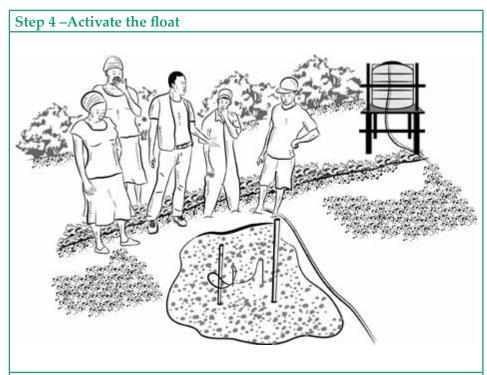
Water the site over the detector after installation to trigger the float. This may require 20 litres or more for a deeper installation.
