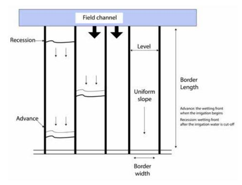
Figure 6.4: Border strips layout (Source: FAO, 2002)
