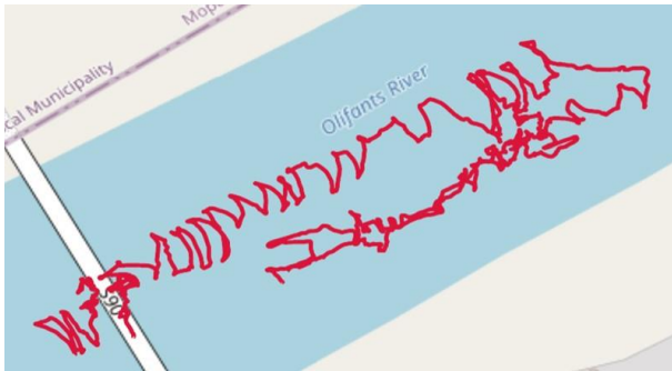
Figure 40 Map view of Bathymetric track covered with HydroSurveyor software.
