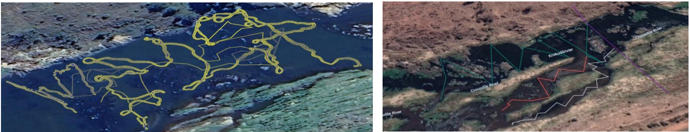
Figure 15 (left and right) Tracks of the River Surveyor generated at the Van Graan Weir on the Crocodile River including the 1D cross-section (purple) and bathymetry (green, red, white) results. Variable direction tracks of the Crocodile River used to generate depth-velocity data for the reach used in the modelling process.
