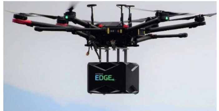
Figure 8 The ASRTALiTe EDGE airborne laser sensor mounted to a DJI M600 UAV.
