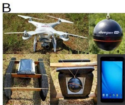
Figure 6 Small UAS-echosounder system. (A) shows the DJI Phantom 3 Pro UAV propelling a mini-boat carrying the single-beam echosounder. (B) shows the DJI Phantom 3 Pro UAV, Deeper Smart SONAR Pro+ wireless SONAR, designed boat and an Android tablet (Diaz et al., 2022).
