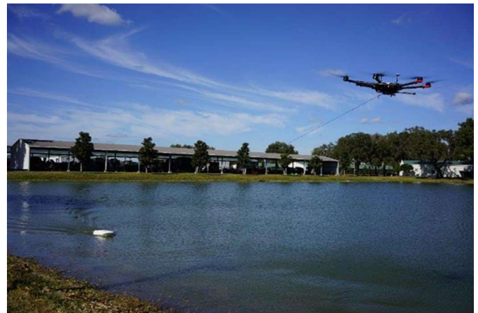
Figure 5 Tethered Bathymetry system which uses a Lowrance Elite ti7 SONAR sensor attached to a DJI M600 drone (Diaz et al., 2022).
