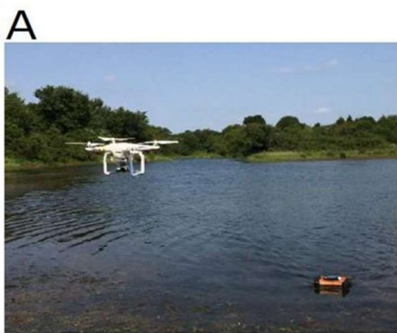
Figure 6 Small UAS-echosounder system. (A) shows the DJI Phantom 3 Pro UAV propelling a mini-boat carrying the single-beam echosounder. (B) shows the DJI Phantom 3 Pro UAV, Deeper Smart SONAR Pro+ wireless SONAR, designed boat and an Android tablet (Diaz et al., 2022).
