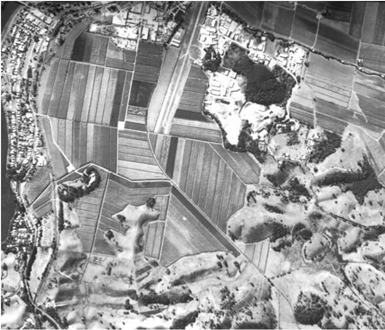
Fig. 9.1. Networks of secondary and tertiary drains on the upper flood plain of the Tweed River, northern NSW, eastern Australia. The river is at far left.
