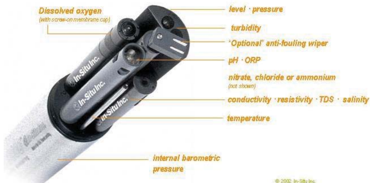
Figure 12. The Troll 9000 in-situ probe used in the monitoring program. Note that not all sensors applied in this study
