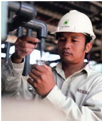
ZERO WATER DISCHARGE: Khun Taleungkiet at the Chachoengsao coffee factory in Thailand, testing the quality of water that has been treated for re-use.
