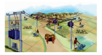
(C) Gujarat's Khushy scheme HVDS with individual minitransformers for farmers anarchy on farm feeder controlled; subsidies and groundwater depletion capped; but at a very high capital cost (MP is experimenting with this)
