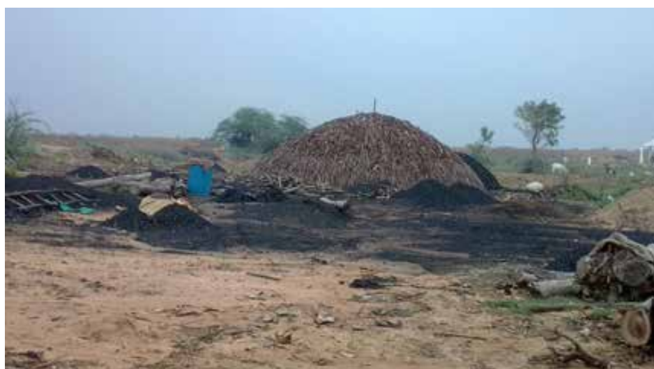
Picture 3: Coal making from the woods of Prosopis Juliflora removed from the tank beds (Picture credits: R. Sakthivadivel)
