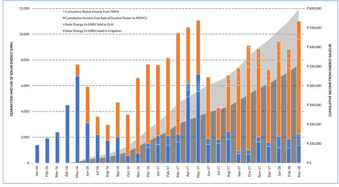
Figure 1: Solar energy generation and its use in irrigation: Monthly data from Dhundi Solar Cooperative
