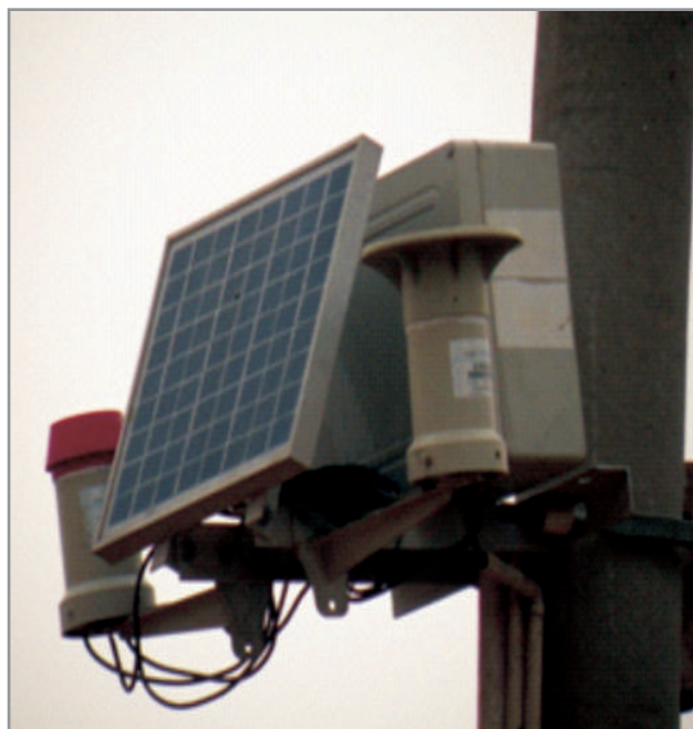
Figure 7 Solar powered groundwater meter transferring real-time water use data to Water Bureau
