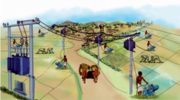
(C) Gujarat's Khushi scheme HVDS with individual mini-transformers for farmers anarchy on farm feeder controlled; subsidies and groundwater depletion capped; but at a very high capital cost (MP is experimenting with this)
