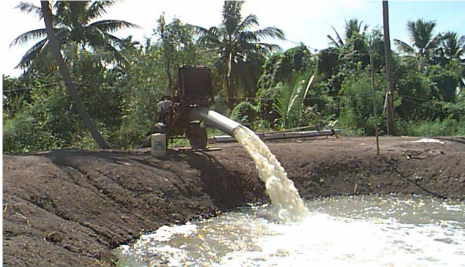
Lift Pump Adding Freshwater to a Low Salinity Shrimp Pond
