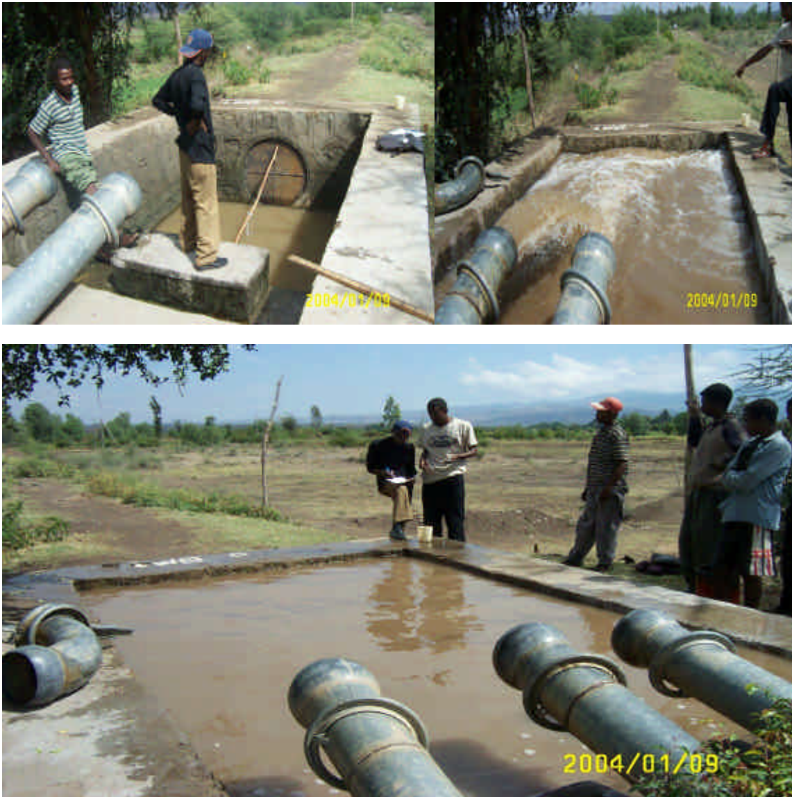
Fig H-5. Discharges of the pumps of Batu Degaga were determined by volumetric method
