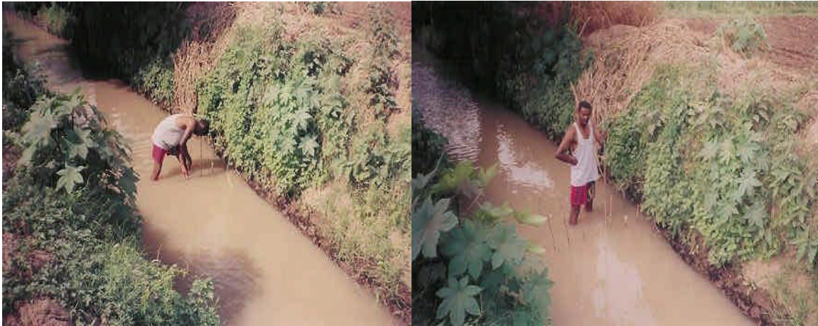
Fig H-6. Discharges measurements of the main canal of Doni was carried out using current meter
