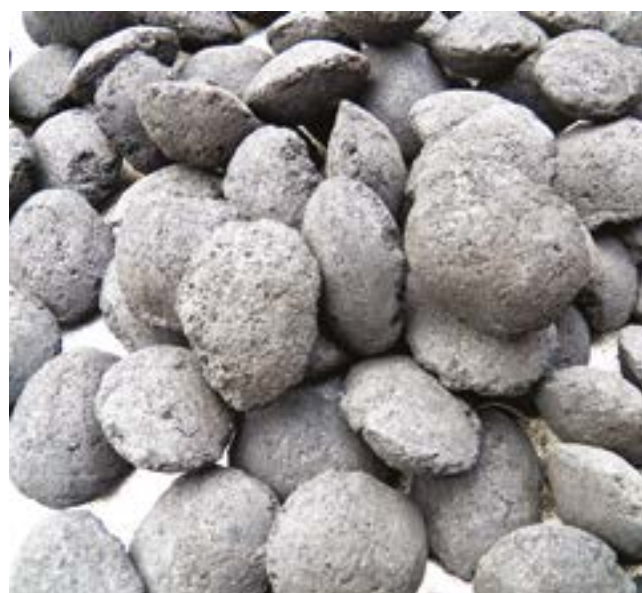
FIGURE 3.1. PILLOW-SHAPED FUEL BRIQUETTES.
