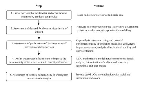
**Figure 15.1** Schematic of Design for Service (DFS) sewage treatment planning framework and corresponding methods
