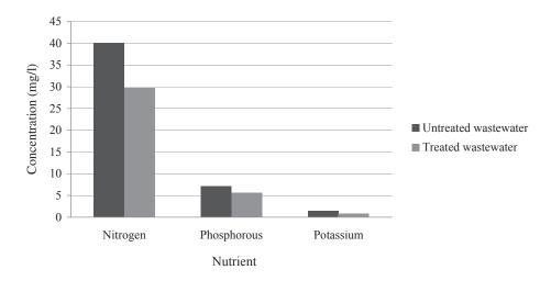
**Figure 6.1** Comparative evaluation of macronutrient concentrations in untreated and treated wastewater from Haryana, India
