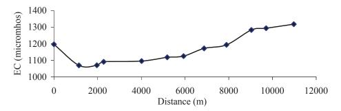
Figure 6.4 Electrical conductivity (EC) with distance downstream of discharge point, Rio Guanajuato, Mexico, 1998
