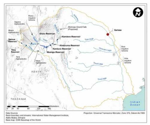
FIGURE 34. Major built infrastructure of the Tana River Basin. As illustrated here, most infrastructure is confined to the upper basin.
