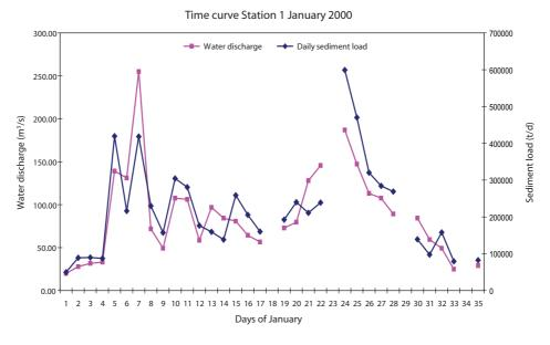
FIGURE 22. Sediment discharge curve at Guder (Bello) station.
