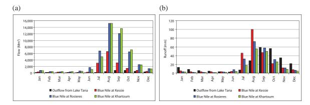
FIGURE 16. a) Mean monthly flow (Mm<sup>3</sup>), and b) runoff at gauging stations located on the main stem of the Blue Nile.
