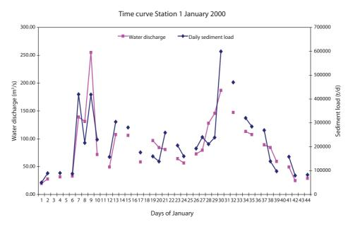
FIGURE 21. Sediment discharge curve at Addis Zemen (Ribba).
