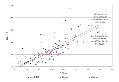
FIGURE 20. Biweekly summed rainfall/discharge relationships for all three watersheds, but only during the latter part of the rainy seasons, after 500 m of cumulative rainfall (P-E) has fallen. Linear regressions are provided for the combined plots: all three together are shown with a solid line and only Anjeni and Maybar (together) are shown with a dotted line.
