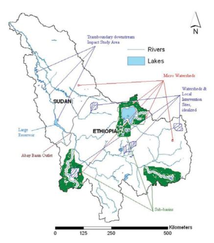
FIGURE 30. Conceptualization of the modeling framework for erosion and sediment modeling across a range of scales.
