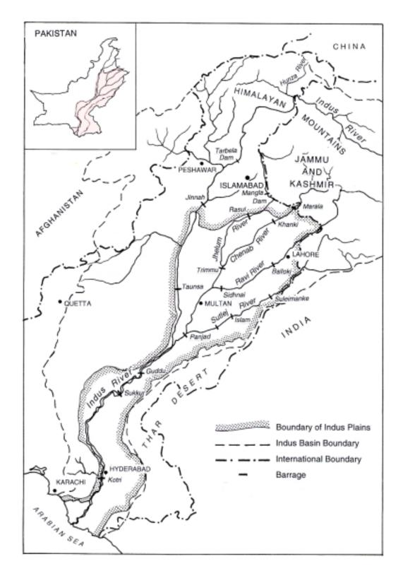
FIGURE 2. Lower Indus Basin irrigation system: Schematic diagram.
