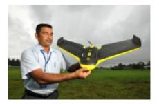
The eBee can spend up to 45 minutes in the air on a single charge of its batteries. Its sensors keep it stable through shifting winds and allow it to avoid other objects that might be sharing its airspace. On completion of mission, the eBee lands automatically, guided by its artificial intelligence module and the global positioning system.
