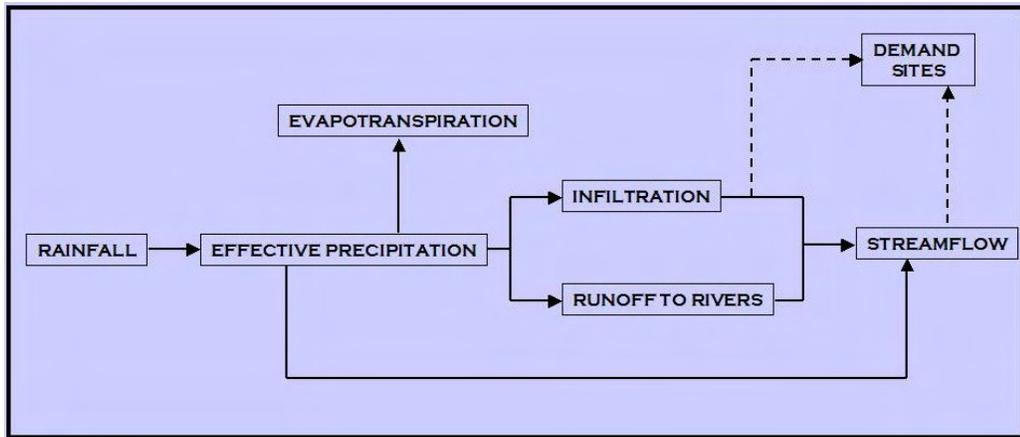
Figure 11 – Schematic of WEAP rainfall-runoff component
