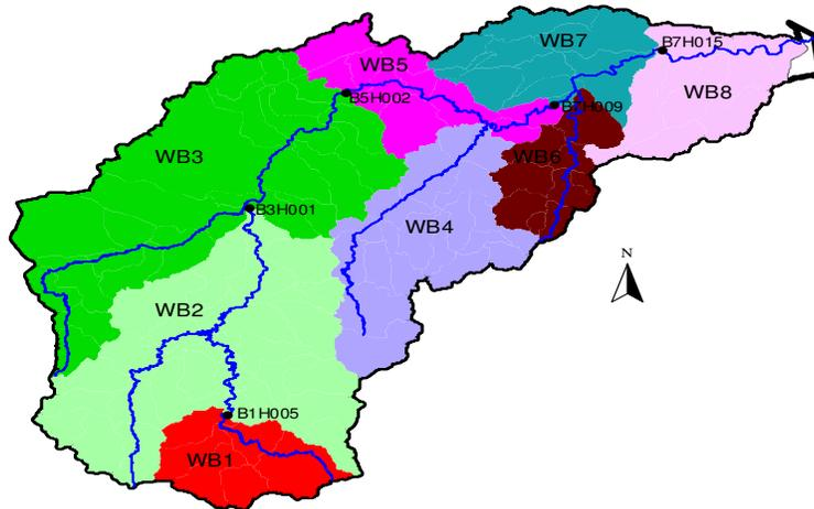
**Figure 9** – Map showing configuration of the WEAP model to simulate flow within eight subcatchments (WB1 to WB8) and the five gauging stations (B1H005 etc) which were used for the model validation.
