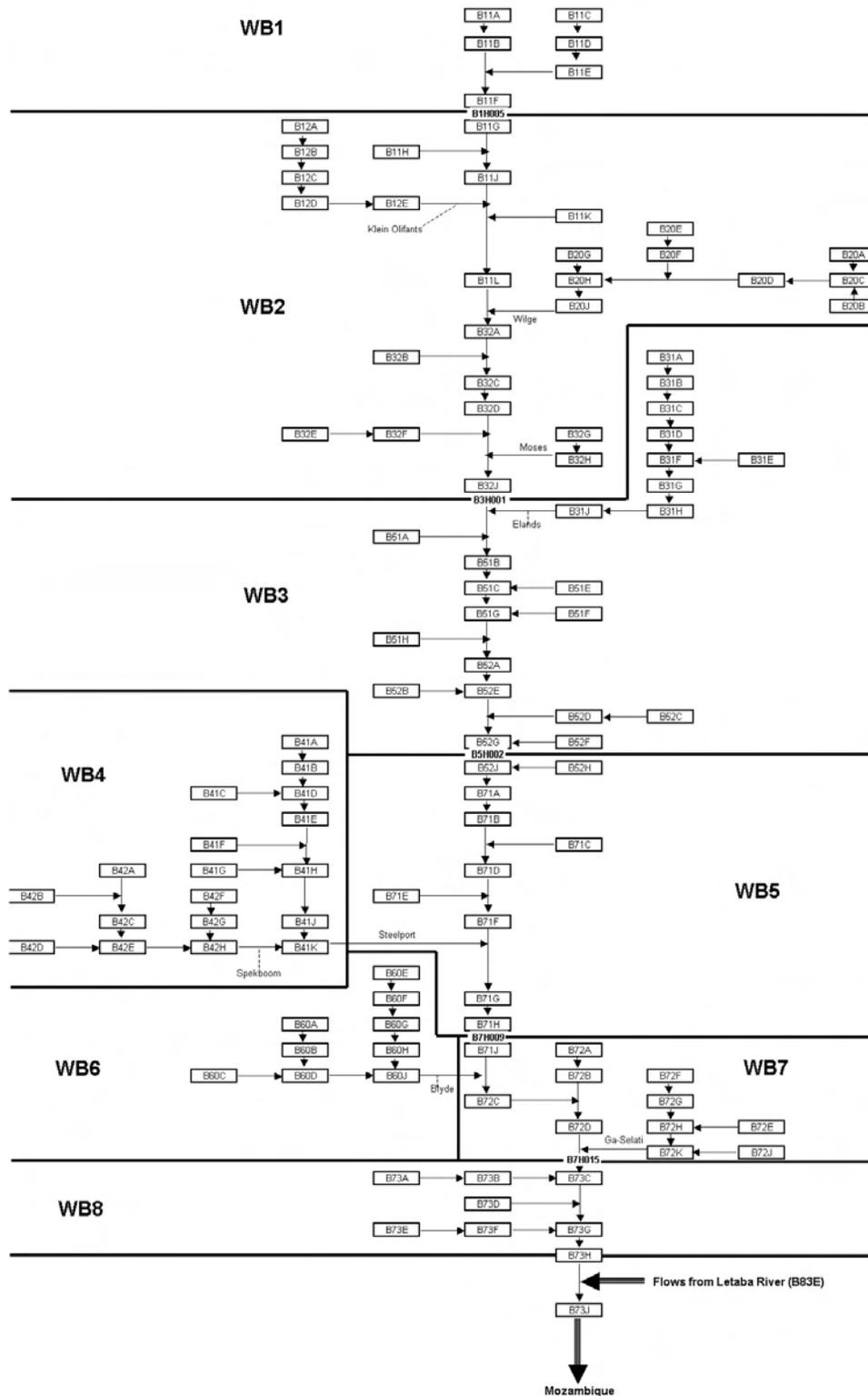
**Figure 10** - Schematic of the quaternary catchments comprising each of the eight WEAP subcatchments.
