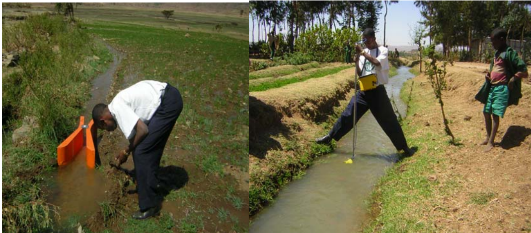
Picture 1. Discharge measurements using current meter and Parshall flume
