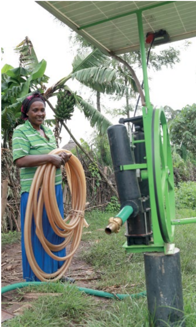
Portable solar-powered pump for irrigation at Jawe community (kebele) in Lemo district (woreda) of Ethiopia's Southern Nations, Nationalities, and Peoples' Region.
